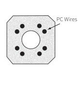
Shaft cross section detail
