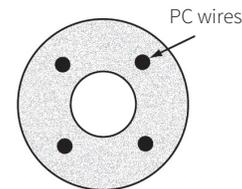
0C2 / 1C2 shaft cross section detail
