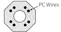
Shaft cross section detail
